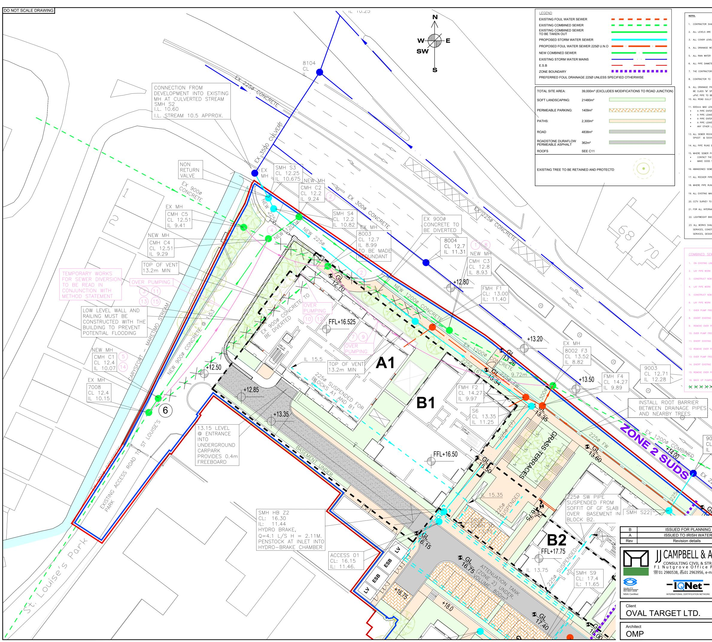
. CONTRACTOR SHALL BE RESPONSIBLE FOR SETTING OUT JUNCTION BOXES, CHAMBERS, MANHOLES, GULLIES TO ENSURE NO CLASHES WITH SERVICE DUCTS AND PIPES.
